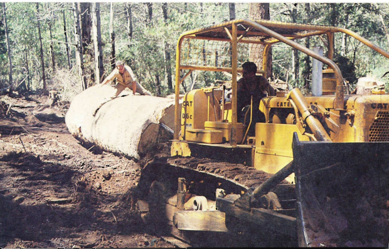
Logging from the hardwood forest—after felling, the trees are cut into required log lengths, snigged to the landing stage, and loaded onto timber trucks for cartage to the sawmill.
